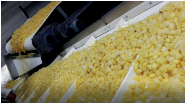
CLINA S20UFMT with transverse cleats conveying potatoes.
