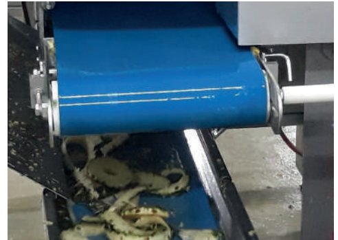
NOVAK S09UF and NOVAK 20CK conveying pineapple residue.
