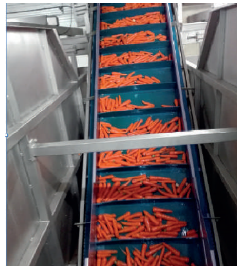
FEBOR 19CK on inclined conveyor with transverse cleats for carrots.
